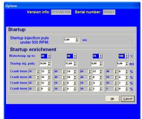
There are four coolant temperature ranges for which an enrichment table can be completed. The additional enrichment (%) in the table can be set during the input of the rpm range. An enrichment map and a startup-pulse can be filled in for four coolant temperature ranges. Above the highest temperature the normal startup pulse will be used.
