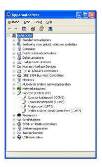
The KMS FA23 system only has an serial port connection. If you want to use this ECU on newer PC's with only USB then you will need an USB to serial converter. In this example on the left (start $\rightarrow$ control panel $\rightarrow$ system $\rightarrow$ device manager) you can see that the USB-to-serial connection has set to COM 7.
