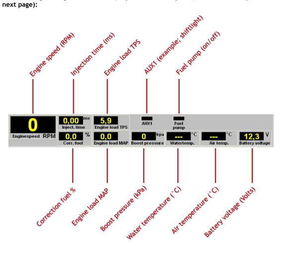
(Boost pressure will change into air pressure, depending on the hardware configuration)
