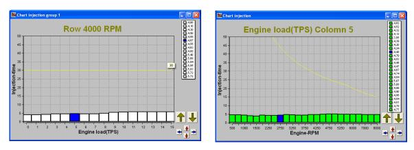
You get overflow of injectiontime when one injection takes more time than the time for two rotations. The time of these two rotations is the maximum injection time because the upcoming rotation is for the next injection.
