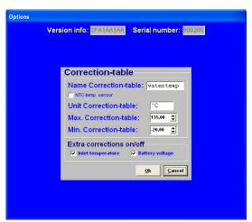
software it does not have to be calibrated. When another sensor is used, the range can be set manually.
