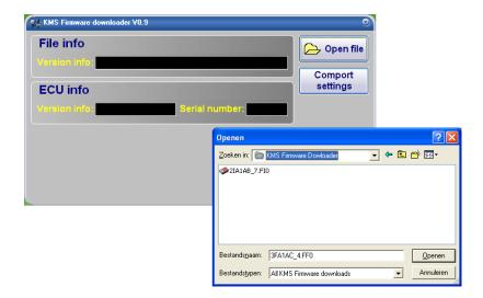
For IA23 the update file name starts with the number 2 and has extension \*.FIO. It's only possible to use this firmware downloader if you have an KMS ECU with serial nr. higher then 300000.
