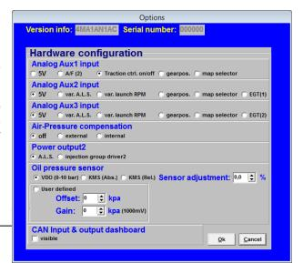
Gearbox position: If gearbox has 0 - 5V position sensor, the signal can be connected to the analog input in order to make variable settings in the powershift and boost control.
