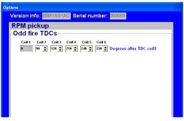
of the block. So the degree for these cylinders isn't on the degree calculated before when deviding 720 dregrees through all cylinders but the angle of the block. The degree for the second cylinder on the same crankpin is the sum of the degrees from the first cylinder on the same crankpin and the angle of the block.
