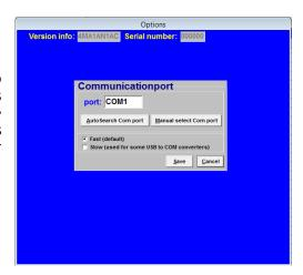
If you choose to use the manual COM port selection it is necessary to look up the correct COM port. Depending on your computer, the used COM port can differ each time the KMS ECU is reconnected. This can be found under your computers 'Device manager' in the 'Configuration screen'. It should be listed in the Port tree containing all COM & LPT connections. In this example you can see that the USB connection has been set to COM 8. Select this port in the KMS Software and press 'Save' to set it.
