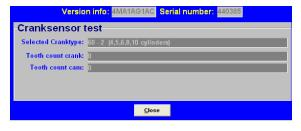
If another reading is shown, check whether the sensor is correctly connected and properly mounted. Electronic interference can occur when the leads are not properly shielded or positioned close to the coil and spark leads. A sensor taking a reading from an external cog may have metal particles attached to it as a result of grinding or drilling. If a failure only starts occurring at higher engine speeds, it is likely that it is caused by sensor vibrations.
