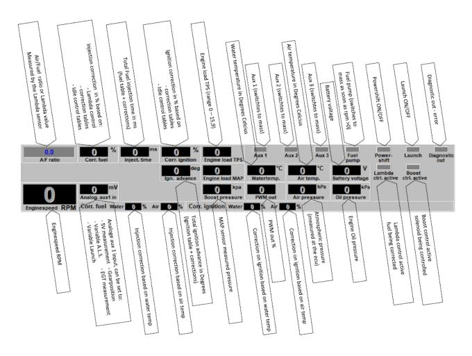
These readings can be used to check whether the right sensors are being used and all settings are correct.
