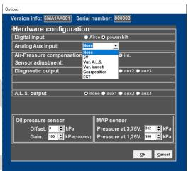
With the Air pressure compensation is set to active (External or Internal) the correction table for Air-pressure in Mbar is active. See <u>Correction tables</u>
