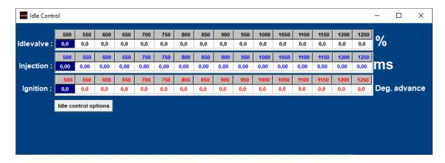
This function (idle-control) will show tables and parameters, where you can adjust the fuelling in ms, ignition in degree advance and opening of the idle-valve in %. (500-1250rpm)
