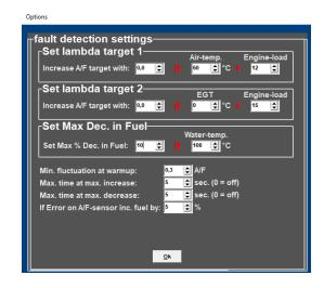
Here you can input a maximum negative injection correction when the coolant temperature exceeds a certain setting. This parameter can be used as protection against engine overheating. If supplementary enrichment has been set in the coolant temperature compensation table for high water temperatures in order to protect the engine, this parameters of this function can help prevent the A/F ratio feedback control from curtailing supplementary enrichment.
