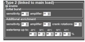
intervene to avoid a short lean mixture. The sensitivity is linked to opening speed of the throttle. A low value for sensitivity means that the initial burst won't occur fast, a high throttle opening speed is needed. For a high sensitivity value a lower throttle opening speed is needed for initial burst enrichment to occur. The amplifier is more or less a factor for the amount of fuel injected. A higher amplifier results in more enrichment.
