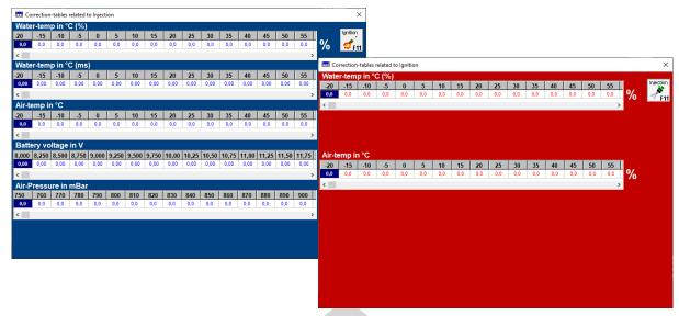
Function key F11 switches between injection correction charts and ignition correction charts.
