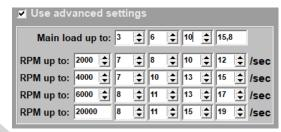
If the sample rate is set too low, the lambda control does not reach the desired target in time. On the other hand when the sample rate is set too high the lambda control will get instable.
